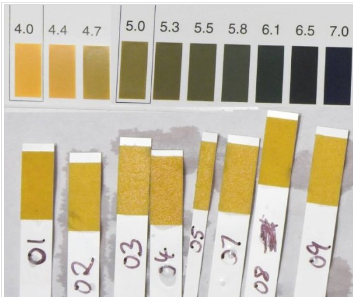
Figure 4 - colorpHast strip after being used in a sample of beer with a pH of 4.40 at room temperature.
