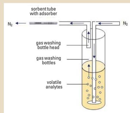
**Fig. 1** Washing bottle with head for extraction of analyte and enrichment on the sorbent tube for thermal desorption
